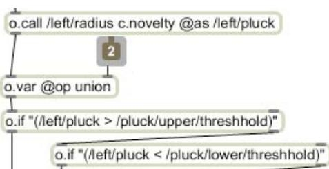
As is typical of these simple detectors the thresholds of detection need to be adjusted using, for example, `o.multisliders` as a source of parametric control:
